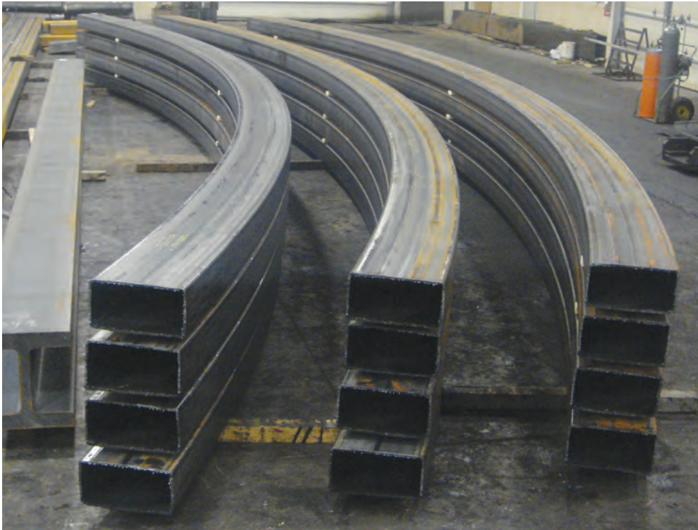
(a) Rectangular HSS bent the hard way
