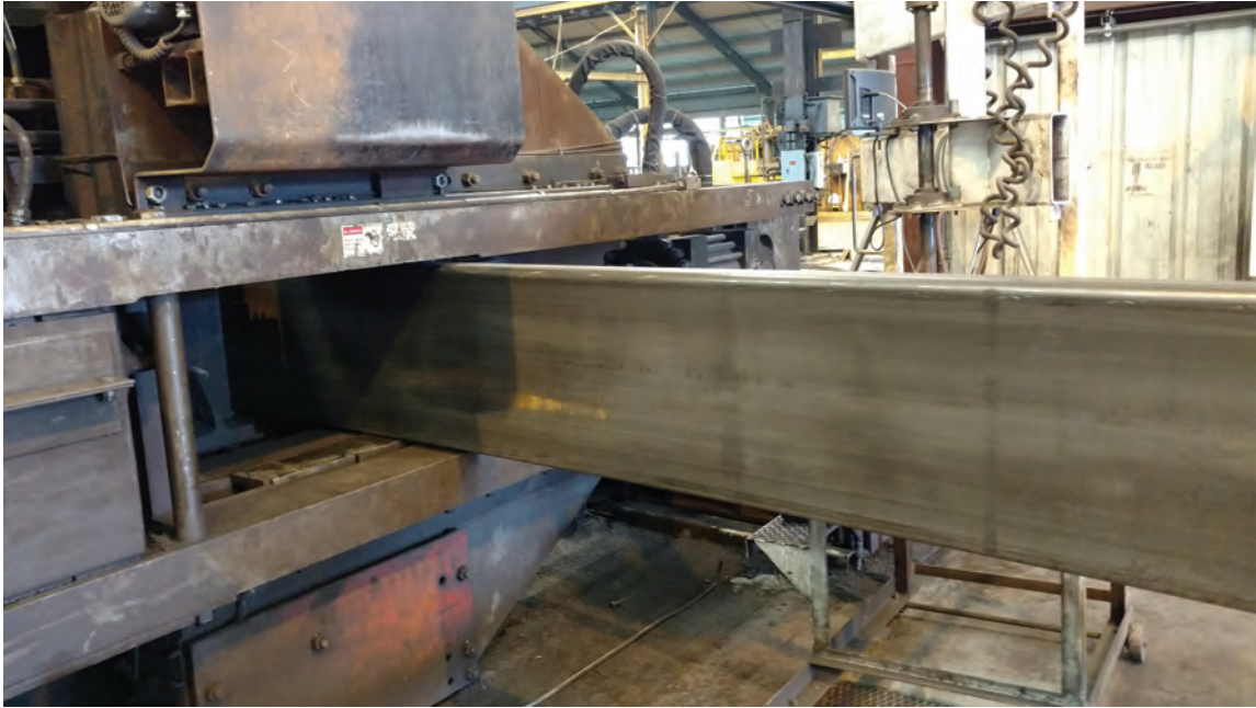
Fig. 2-15. Incremental step bending of a rectangular HSS (courtesy of AISC Bender/Roller Committee).
