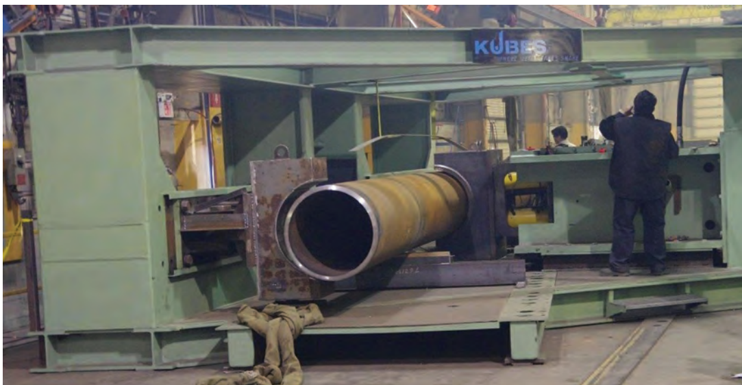
Fig. 2-19. Ram bending of a round HSS (courtesy of AISC Bender/Roller Committee).
