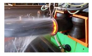
"Our induction bending capabilities allow us to provide customers in need of distortion-free bent tube, pipe or structural shapes with an exceptional product," said Joe Wendt, president of CMRP. "Induction bending is one example of how our company is evolving to meet the growing needs of our customers. Adding induction bending to the breadth of our capabilities, coupled with our highly skilled workforce, helps makes us a trusted bender roller for customers across the nation."
